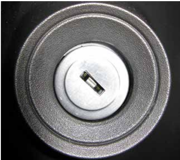
Photo 10. Close-up view of sidebar ignition lock in a 2008 Cadillac CTS. Notice shutter assembly across front of keyway.
