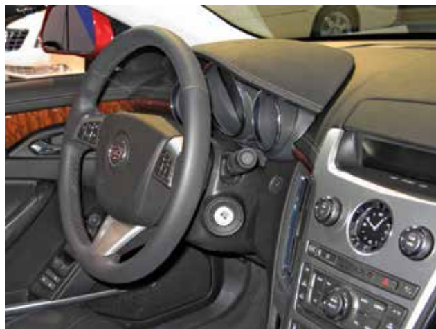
Photo 8. Steering column of a 2008 Cadillac CTS equipped with sidebar ignition.
