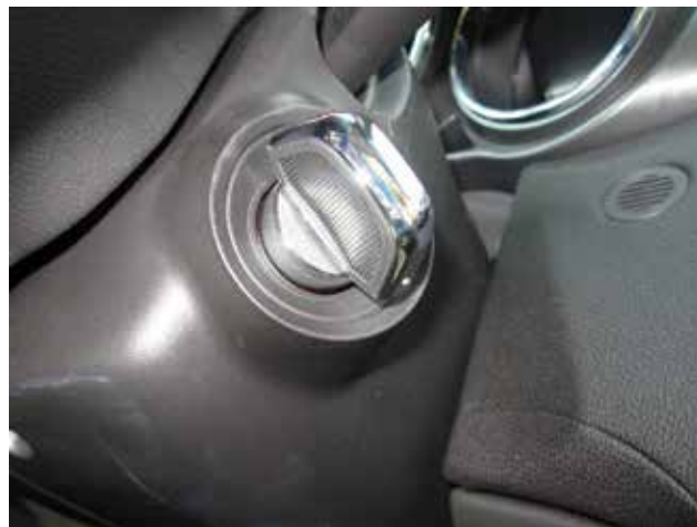
Photo 9. The turn-knob on a 2009 Cadillac CTS equipped with the proximity fob option -- no ignition lock.
