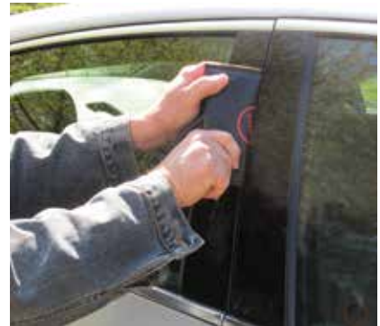
Photo 6. Air wedge in place
