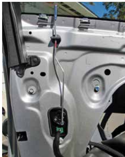
Photo 2. Vertical linkage rod sandwiched between inner door skin & trim panel
