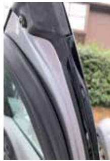
Photo 4. Thin wrap-around metal trim
