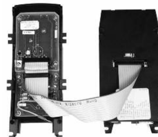
Ribbon Cable Orientation: Install with cable exiting DOWN, as shown.
