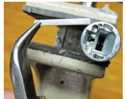
21. Tumbler retainer removed from lock
