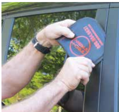
2. Because of the stiffener inside the air wedge, the Tech-Train air wedge can be inserted without using a lever to enlarge gap
