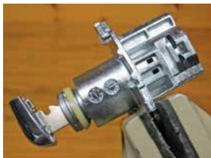
13. With clip removed and plug turned a quarter turn, pull the plug free of the housing
