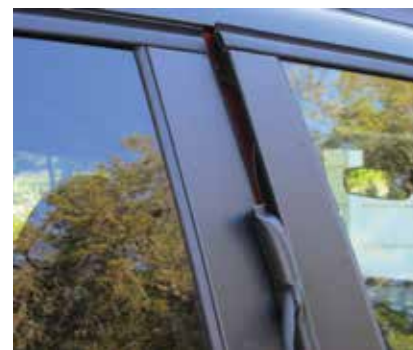
3. Air wedge can be inflated to give a large enough gap between door & frame to insert the opening tool
