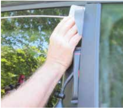
4. Long-reach rod inserted through the opening into the vehicle using the finish protector sleeve to keep the rod from touching the painted surfaces of the door and door frame
