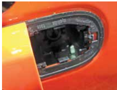
8. One of two lugs of the clamp assembly that secures the door lock in the retracted position where the lock can be removed
