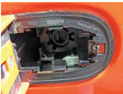
7. One of two lugs of the clamp assembly that secures door lock in the secured position
