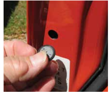
6. Lock secured into the door with a clamp assembly that can be accessed by removing the rubber plug on door edge
