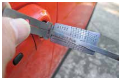
24. SIP-22 Lishi tool in use to decode the lock after picking it
