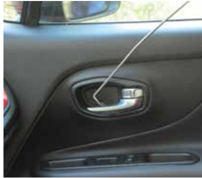
5. Inside view, tip used to lever the inside handle out, which will override the lock system and unlock the door
