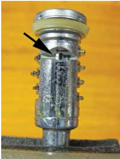
16. Arrow points to portion of tumbler retainer visible inside one of the shear points on the plug (Shear points are intentional weak spots in the plug so that the plug will break rather than unlock the vehicle if it is force rotated)
