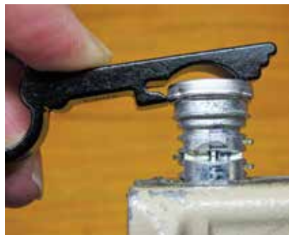
17. Keychain-style bottle opener used to remove face cap from plug
