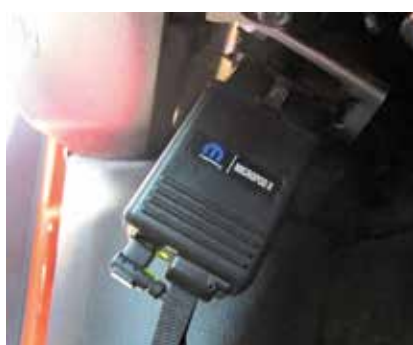
26. "Micro Pod" tool in use plugged into the OBD II port
