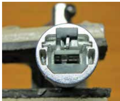
20. Tumbler retainer now visible in cavity below face cap
