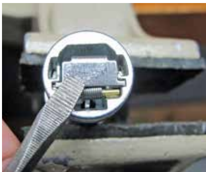
19. Shutter components that are held in place by the face cap
