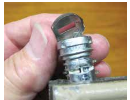
18. Face cap being lifted free of plug
