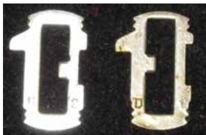
23. Close-up of a tumbler from each side of the lock showing the number and letter stamps
