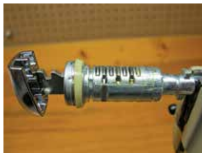
14. Lock plug contains seven tumblers in positions 2 – 8
