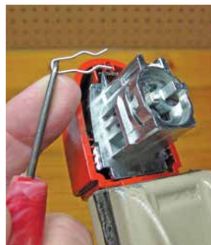
12. Spring clip removed from the lock
