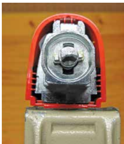
10. Two lugs on rear of plug must be aligned with the slots in lock housing to remove lock plug
