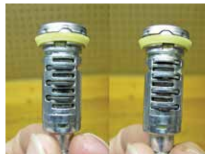
15. All of the springs are located on one side of keyway
