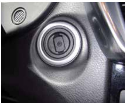
Photo 17. Slot in the dash of Infiniti QX30 is for a typical Mercedes-style FOB.
