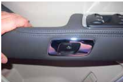
Photo 19. To exit the vehicle, you must press the button recessed into the armrest.
