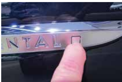
Photo 20. Continental emergency door lock cylinder concealed in trim along forward edge of driver's door
