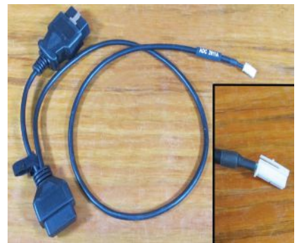
The ADC2011 cable is necessary to program the 2018 Chrysler 300 and some other Chrysler vehicles. The end that plugs into the vehicle is shown in the inset.
