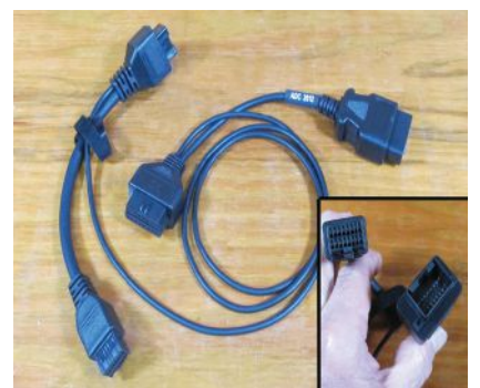
The ADC2012 cable is required to program certain Fiat Chrysler Automobile vehicles. The end that plugs into the vehicle is shown in the inset. It has a male and a female Star connector and is inserted between the two connectors in the vehicle.
