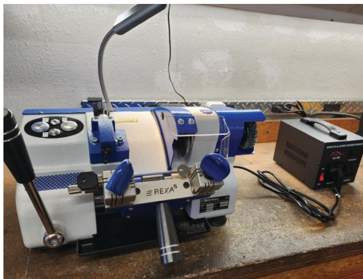
Photo 2. The Börkey Rexa 5 has a LED indicator light that engages when the depth adjustment button is pressed.
