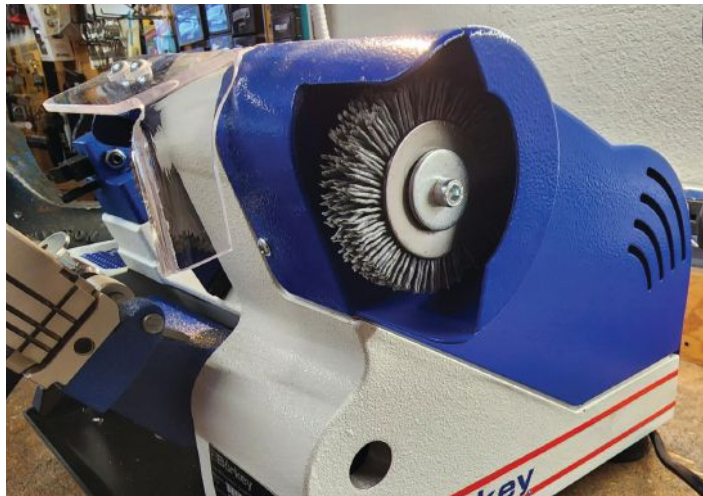
Photo 3. Built-in plastic brush for easy buffing of completed keys
