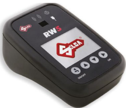
Photo 2. The RW5 is significantly smaller than previous RW cloning devices
