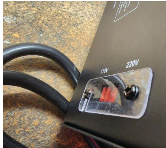
Photo 5. Check the voltage selector setting switch on the back of the power supply
