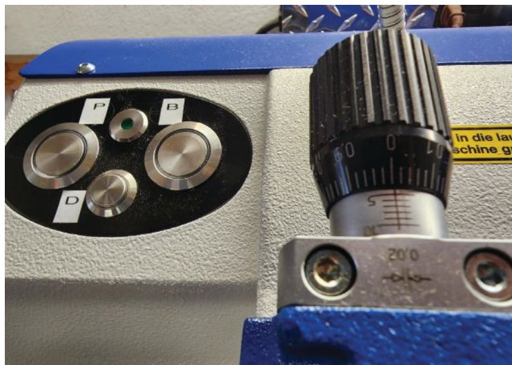
Photo 1. The Börkey Rexa 5 has a LED indicator light that engages when the depth adjustment button is pressed.
